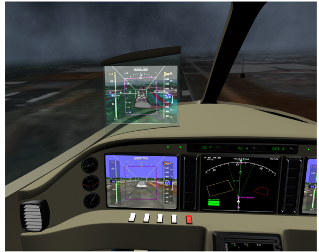
Fig. 7 Advanced cockpit concept utilizing a PFD with HITS flight-path guidance, a MFD with navigational tools, and HUD for out-the-window monitoring for improved flight-path accuracy and situation awareness in IMC.
