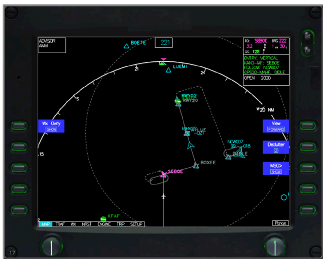
Fig. 4 Multifunction display showing HVO functionality to the pilot.
