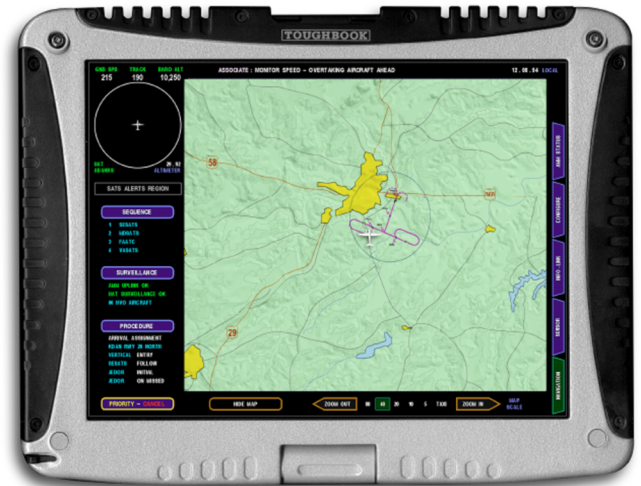
Fig. 15 Virginia SATSLab electronic flight bag provides the pilot navigational information and HVO functionality to allow for increased situation awareness and performance.
